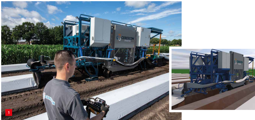
Remote control of the Sparter by an operator. The inset shows the handling of the plastic foil. At the row entrance, the operator puts the foil in the machine; then further along the row, the Sparter picks it up and places it back on the bed at its rear.
