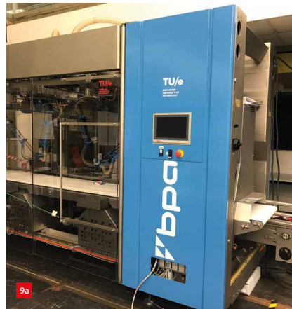
A BPA spider twin delta robot installed at TU/e for research and demonstration purposes in the food-packaging use case.
