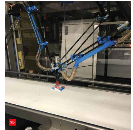
A BPA spider twin delta robot installed at TU/e for research and demonstration purposes in the food-packaging use case.
