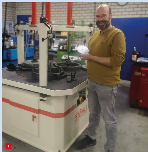
Nobby in front of his largest lapping machine, with a lapping disk of 1 m.
