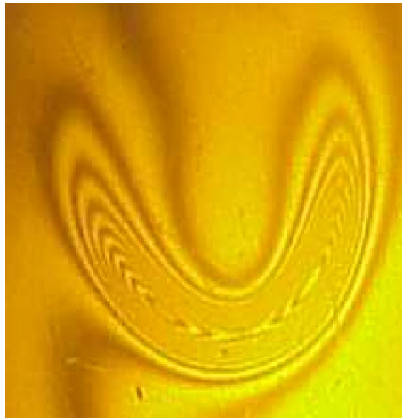
Figure 6. Verification of the final result shown in Fig. 5. The Newton fringes in sodium light are shown as obtained by placing the work piece on a flat reference sample.
