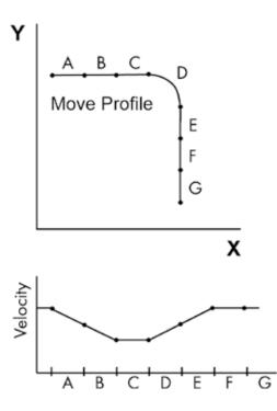
Figure 3. Contoured motion is facilitated by the multi-block lookahead feature, which allows the controller to anticipate sharp corners and small radius arcs and automatically accelerate and decelerate as needed.
