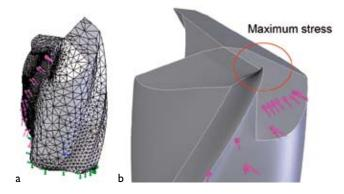
Figure 3. Study of tool geometry by FEM.
