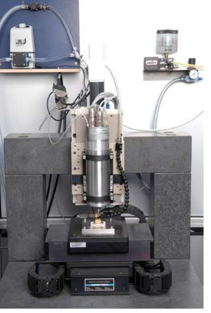
Figure 8. Micro-milling setup at Delft University of Technology, with an AMB spindle with max. rotational speed of 120,000 rpm.
