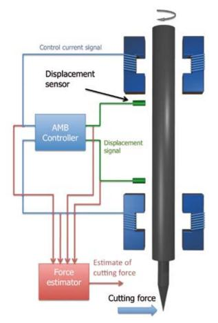
Figure 6. Schematic illustrating the concept of cutting force estimation with an AMB spindle. Cutting forces acting on the tip of the endmill can be estimated from the closed-loop current and displacement signals of the magnetic bearings.
