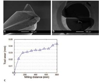
Figure 2. Wear of tested commercial  $\emptyset$  0.5 square endmills. (a) 3D view.
