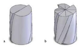
Figure 4. Cutting part of newly-designed micro-endmills. (a) 2-flute endmill. (b) 4-flute endmill.
