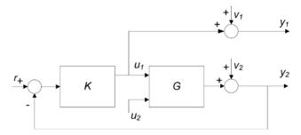
Figure 7. Block diagram of the closed-loop AMB spindle system. Cutting force estimation can be formulated as an input estimation problem, where the forces are the unknown input  $u_2$  to a partially closed-loop system consisting of the AMB spindle dynamics G and controller K.
