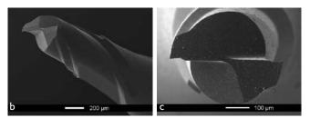
Figure 1. Geometry of a micro square endmill.
