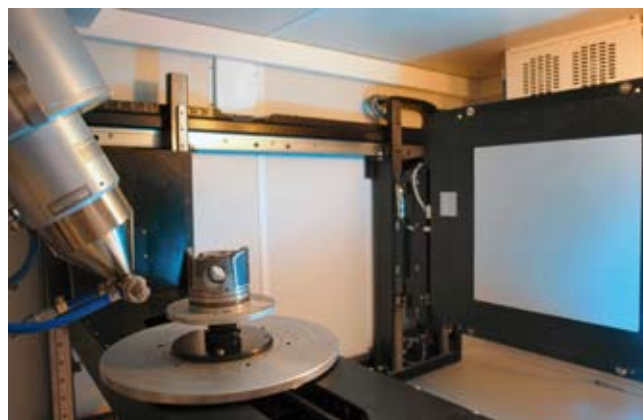
Figure 4. The Nikon Metrology 225 kV Ultrafocus X-ray source (left) and the silicon flat panel-detector Varian 2520 (right) with a piston as the object to be inspected.
