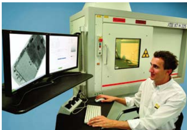
Figure 3. Working with the Nikon XT H 225 CT measuring machine.
