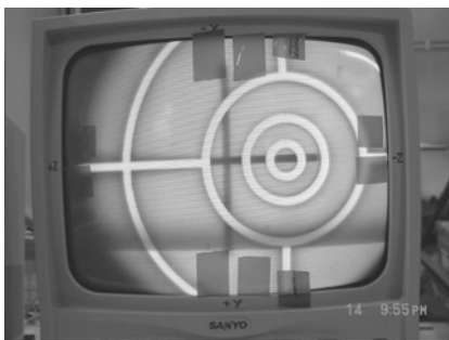
Figure 17: Shift of VIS system recticle with respect to central marker (black) of calibrated plate due to diaphragm plate cool down from +20 °C to -188 °C.
