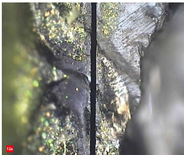
12a Waterjet-guided laser technology. (a) Straight diamond cut. (b) Synova's Laser MicroJet in action.
