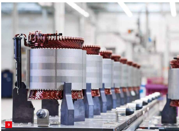
BMW e-motor manufacturing line recently opened in Dingolfing (Germany), at the top of each motor showing the protruding ends of hairpin-like windings that are laser-welded together.
