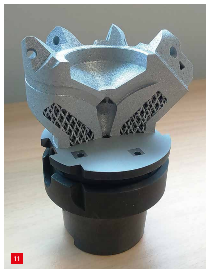
3D Systems presented examples of tooling that were produced by hybrid manufacturing, combining the machining of the base block and the printing of the tool head.
