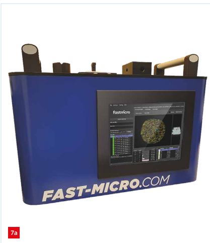
Cleanliness was measured with the Fastmicro Sample Scanner using PMC cards (right).
