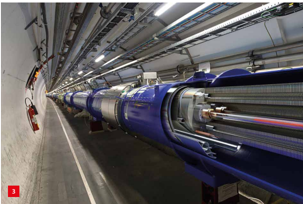
3D cut of the Large Hadron Collider dipole at CERN. For ultra-high vacuum and cryogenic application, suitable materials had to be selected for, e.g., beam pipes, heat-exchanger tubes, magnetic inserts, iron yokes, non-magnetic collars and superconducting coils. (Image: Daniel Dominguez, CERN)
