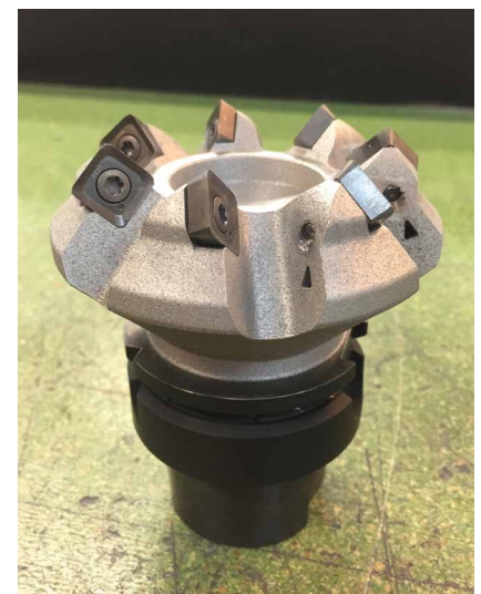
3D Systems presented examples of tooling that were produced by hybrid manufacturing, combining the machining of the base block and the printing of the tool head.
