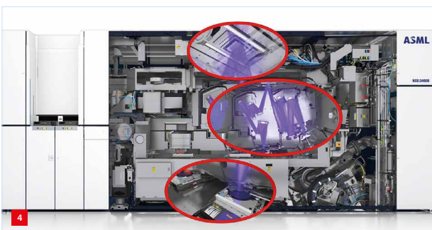
Critical contamination areas in an ASML EUV lithography machine, from top to bottom: reticle, optics, wafer.
