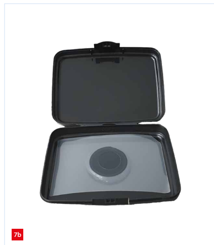
Cleanliness was measured with the Fastmicro Sample Scanner using PMC cards (right).
